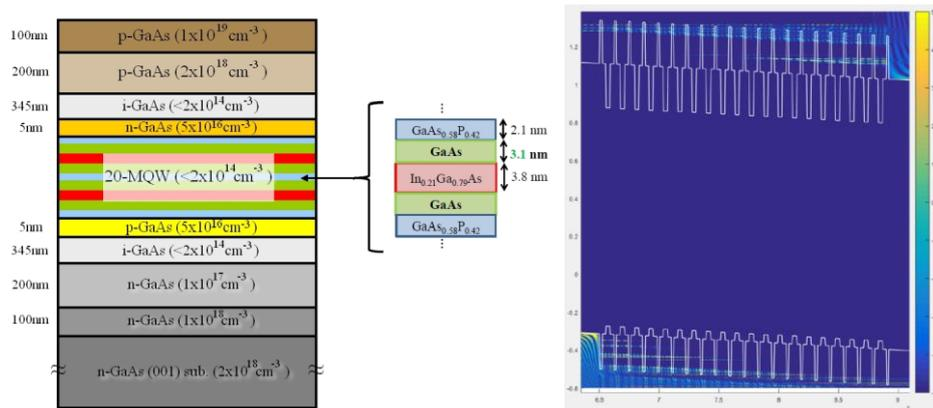
Figure 1. Schematic representation of the cell considered in this work and the local density of states versus position and energy obtained in the MQW. This last result exhibits minibands in both valence and conduction bands.
