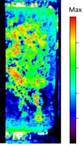
Encapsulated cell after aging at 85°C/85%RH
