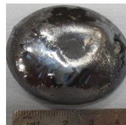
Figure 2: picture of an ingot obtained after melting of kerf-loss Si powder.
